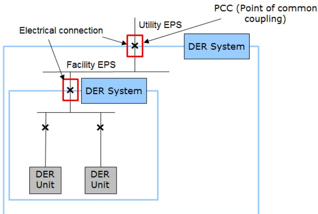
Figure 3: The concept of a DER system
