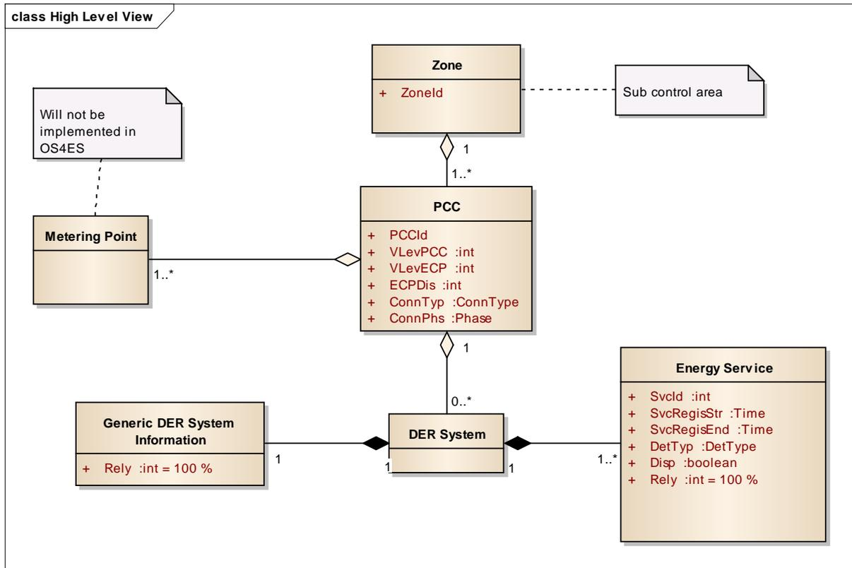
Figure 5: Embedding of the DER system in the electrical network structure
